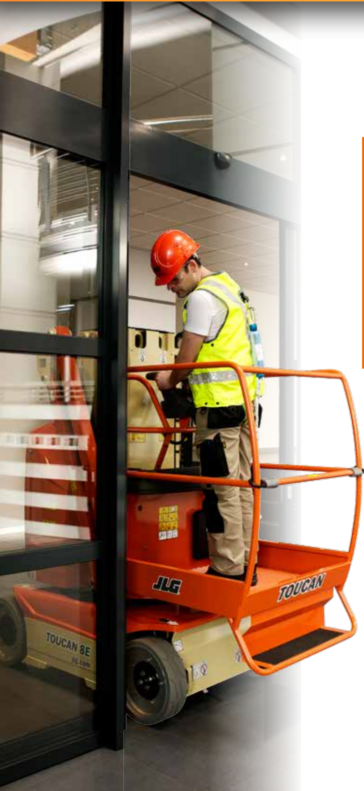
The Toucan 12E Plus is equipped with basket rotation.
